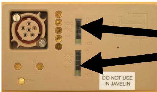
These are the indicator bars. The dark bars reflect the amount of charge in the battery. Five black bars mean the battery is fully charged. When no black bars are present, the battery is empty. The battery in this picture shows a battery with just under a full charge.
